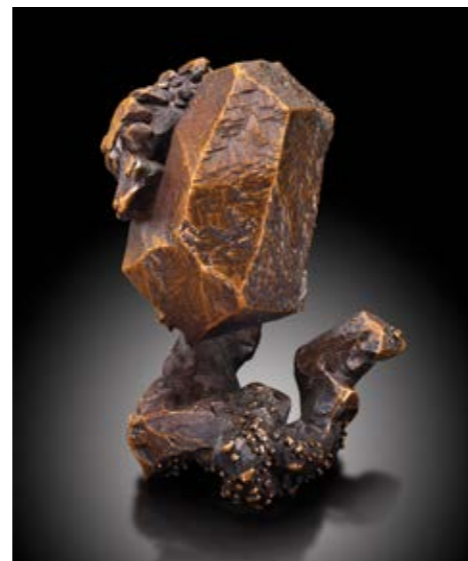
Copper. Keweenaw County, Michigan, USA. 8 x 7 x 6 cm, mim specimen #1125: Pure crystallography which we can observe in this huge native Copper crystal, with its well-defined faces and edges, an elongated tetrahedral morphology, with the edges very distinct due to their more ochre color while the faces of the crystals exhibit a darker color due to a patina. Accompanying this dominant crystal are small copper crystals, giving even greater gravitas to this specimen. For crystal sharpness and crystal size, it is an unbeatable Copper. James Elliott Photo
