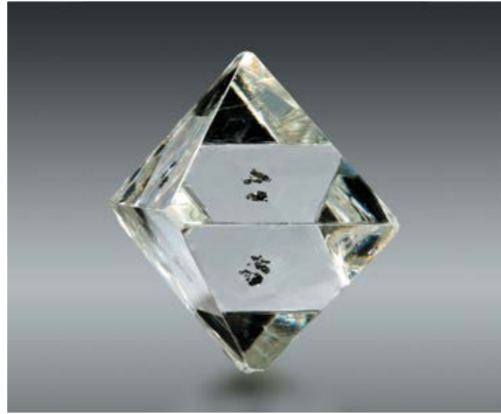
Diamond. Udachnaya-Vostochnaya pipe, Daldyn, Daldyn-Alakit, Sakha Republic (Yakutia), Russia. 2.5x1.9x 1.9 cm, mim specimen #1591: This diamond specimen represents the epitome of the cubic system. A perfect octahedron with smooth and flat faces and very sharp edges with sulfide inclusions - probably pyrrhotite and pentlandite. The fact that this specimen does not exhibit rounded faces indicates that the kimberlite that hosted it had an extremely fast vertical rise towards the Earth's surface. A diamond that is not at all boring, thanks to the inclusions it exhibits. James Elliott Photo
